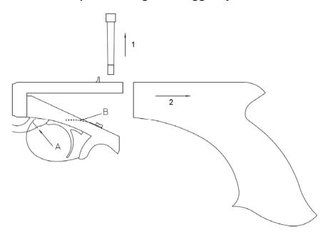
A = trigger adjustment screw B = trigger spring
